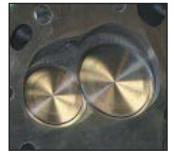
Highly efficient combustion chamber and big 2.080" intakes
