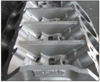
Reinforcing ribs provide improved bank-to-bank stability and indexed lifter bores assure optimum valve tain operating efficiency.
