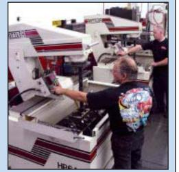
One of the key operations in race-prepping a block is honing the cylinders to the desired specifications using special plates to simulate the loads exerted on the block by the cylinder heads. World employs highly accurate Rottler Power Hones for the task.
