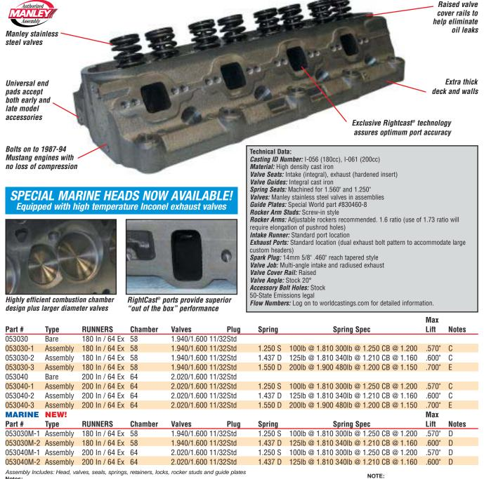
Notes: C = 7° Stamped heat treated steel valve locks, Manley 4140 chrome-moly retainers and Nitrile umbrella seals 50 State Emissions Legal: Important note: Windsor Jr./Sr. cylinder heads carry D = 10° machined steel valve locks, Manley 4140 chrome-moly retainers, Nitrile umbrella seals and Inconel exhaust valves (Marine version) C.A.R.B. EO #D-343-1 E = 10° machined steel valve locks, Manley 4140 chrome-moly retainers, Teflon seals and Manley Race Master valves
