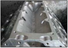
The Warhawk' block is designed with priority main oiling so the bottom end gets fed first and "upstairs" last
