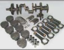
SHORT BLOCK KIT AND ROTATING **ASSEMBLY - Kit** contains a raceprepped Motown II iron block and an internally balanced rotating assembly with 4340 crank, H-beam rods, forged pistons wrist pins, piston rings, plus rod and main bearings
