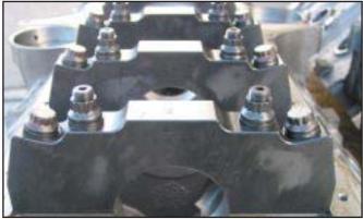
With 4-bolt splayed 1045 alloy billet steel main caps and 200,000 psi ARP® main studs and bolts, superior reliability is assured.
