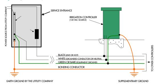
Vac power sources, the wires are Black, White and Green. For 240 Vac power sources, the wires are Black, Red and Green. Power wires must always be kept together in a trench, conduit, tray, etc. The bonding conductors are required to be 6 AWG solid bare copper, unless the system power conductors are larger than 1/0 AWG, in which case the bonding wires are to be 4 AWG solid bare copper.
