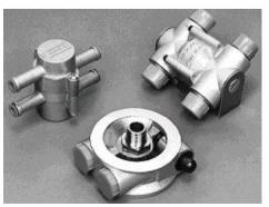
The oilstats should only be used where oil cooling is adequate, the wax element will suffer permanent damage above 140°C, replacements are available.
