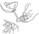
STEP 5. Lubricate inside of hose and nipple threads liberally using S.A.E. 30 lubricating oil.
