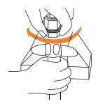
STEP 6. Carefully insert nipple and engage nipplé and socket threads while holding hose in position with other hand. Make sure hose does not push out of socket by observing mark made in step 3.
