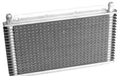
The PWR range of 19mm deep coolers is of aluminium pressed plate construction, they are configured to suit cooling systems powered by electric remote pumps with their lower oil flows than engine driven pumps. Compared to our range of 50mm deep coolers their narrower oil passages offer higher oil flow resistance but this is of
