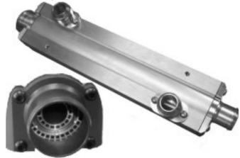
Provides engine oil cooling for more demanding applications. Construction is similar to C43 range except oil outlets are parallel not on opposite sides. Available with twin oil side cores, one fitted inside the other. Heat transfer for the twin core example is almost double the C43-330. Currently available with oilside connections in -8, -10, -12 & -16 SAE 37 $^\circ$  (JIC) and waterside to take 28, 32, 35, 38 and 45mm bore hose.
