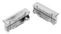
Construction. Aluminium die casting with angled pockets to hold any size hexagon and horizontal pocket to hold all sizes of hose. Cast in magnets hold jaws firmly to vice. Application. Holds anodised fittings during assembly minimising marking the finish and allows hose to be held firmly during cutting operation.
