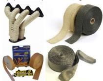
Application. It is widely claimed that insulating the exhaust manifold pipes will produce more horsepower, it will certainly reduce under bonnet temperatures with consequent benefits. Daily use may lead to more rapid corrosion of thin section manifolds. Secure with stainless steel cable/hose ties.
