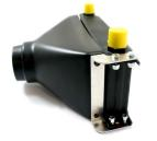
High quality oil cooling air ducts have been specifically designed to mount quickly and easily to 13, 16 or 19 row Mocal or Setrab type oil coolers. Supplied with laser cut aluminium mounting brackets and all fittings. The main body is formed from HDPE. Stepped inlet to accomodate two sizes of ducting 63/76mm on 13 &16 row. 19 row duct designed with double inlet 76/63mm. Oil cooler not included.
