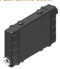
This has a smaller front of 40mm as opposed to the 50mm of the Mocal and STD coolers. Pressure drop will be higher, they are suited for most oil cooling applications but only the 14 row height should be considered for the higher flows found in engine coolong installations. These tube and fin coolers are "Nocoloc" brazed and have a black epoxy finish.
