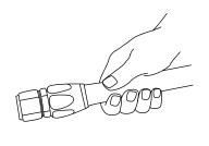
STEP 8. IMPORTANT - Check hose for push out by observing hose position mark. None should be evident.
