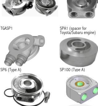
Variations of the SP1 are the OTSP1 with built in thermostatic control the TGASP1 with a tapping for temperature gauge, the SP100 made from billet which fits the Japanese micro filter and the OTSP1HF a thermostatic plate which although bulkier and more expensive offers minimum flow obstruction.
