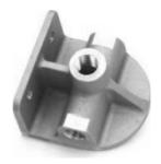
Takes unique Chevrolet filter, big and small block V8s to 1978. 13/16UNF thread and 4" diameter. Left hand in and either top or right hand out, tapped 1/2NPTF. Spare port can be temp or pressure take off
