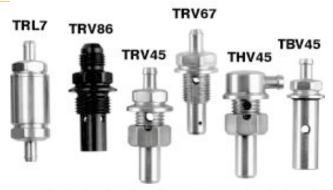
A range of fuel tank valves that allows air in to replace fuel used, air out due to heat expansion and a positive shut off to prevent fuel escape, due to splashing or even roll over. This is achieved by a two ball system, one hollow plastic, one solid steel.
