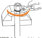
STEP 4. Spanner tighten hex until clearance ith socket hex is 1/32" or less. Tighten further to align corners of nipple and socket hexes. To disassemble: Unscrew and remove nipple; slide socket back on hose by tapping against a flat surface, remove sleeve with pliers.
