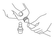
STEP 1. Cut hose to required length with a sharp knife. Oil inside of hose and outside of nipple liberally.
