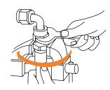
STEP 7. Screw together by hand, then lightly grip socket in a vice. Use a spanner to fully tighten the fitting.
