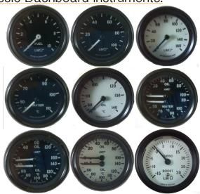
A superb range of high quality 52mm diameter mechanical instruments with precision machined brass movements. Available with white or black face, black, 12 volt back lighting is standard. Temperature gauges have 7 foot (2 metre) capillary tubes with 3/8BSP male connections. Pressure and boost gauges have standard 1/8BSP coned male connections, lines may be either stainless steel braided TFE, see page 38, or nylon as below. For T pieces and adapters to facilitate gauge fitting see page 23.
