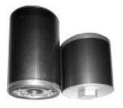
Billet aluminium bodies in two lengths  $4.25^{\circ}$  &  $6.25^{\circ}$  overall x 3" width with threads to fit all popular engines, see chart page 20,to take CM's synthetic fibre 8 micron filter(road) or stainless steel 40micron filter (race). Cleaning of steel filters as XRP.
