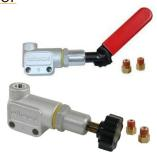
Place in any hydraulic circuit to reduce pressure, maximum reduction 57%. Normally positioned in line to rear brakes, but can be positioned anywhere to produce weird and wonderful effects e.g. on inside front wheel on oval tracks. Aluminium and steel construction. Available with handle giving 7 positive click settings or knob to allow even finer adjustment. Weight 8 oz.
