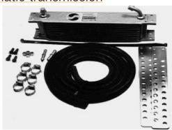
Automatic transmission oil cooler kits are designed for fitting an oil cooler behind the front grille usually in front of the water radiator, brackets are provided to enable the use of the water radiator mounting bolts to secure the cooler. Kits come complete with a cooler, textile braided hose plus all the necessary clamps, nuts, bolts etc.
