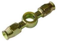
Has slimmer profile than standard banjo. Direct fitting into calipers, wheel & brake cylinders. Takes short banjo bolts see page 57 & 67 for bolts and washers.
