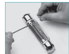
3. Adjust tension; then insert stop pin in hole of adjustment bushing assembly.
