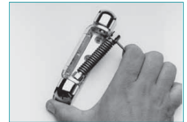
2. Place thrust washer and bushing over hexagon pin on mounted hinge. Insert adjustment pin into adjustment bushing assembly. Grasping adjustment pin, compress spring and place adjustment bushing assembly over round pin.
