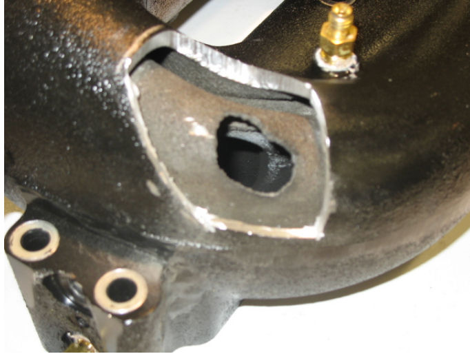
Figure 15: Exhaust Manifold Failure
