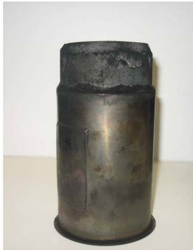
Figure 17: Failed Catalyst From WOT Test
