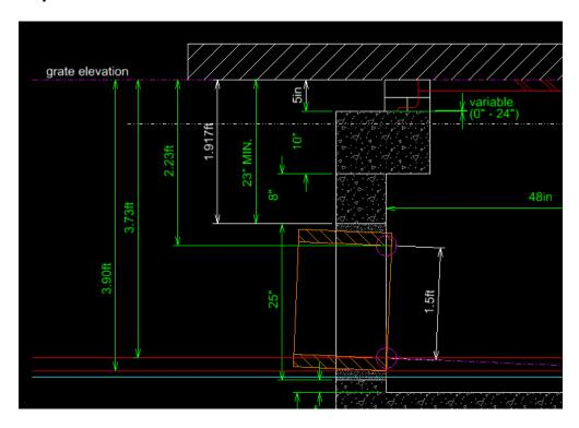
The depth of cover is the vertical distance from the grate elevation to the point where the inside diameter of the inlet pipe intersects the inside edge of the catch basin wall, signified by the upper left purple circle.
