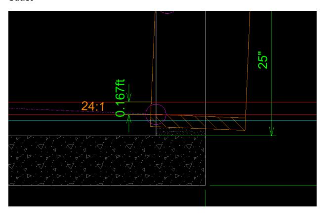
The outlet point of the catch basin is where the inside diameter of the outlet pipe intersects the inside edge of the catch basin wall, signified by the purple circle.
