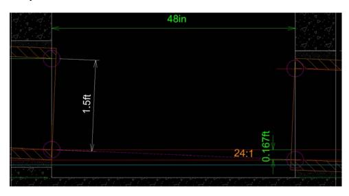
The drop is the vertical distance between the inlet elevation and outlet elevation.
