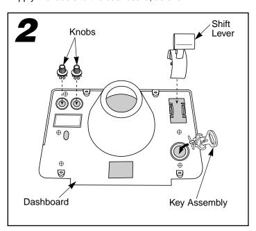
Insert and snap the shift lever, key assembly and knobs into the dashboard, as shown.
