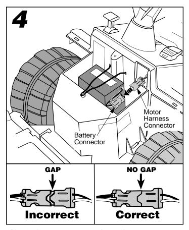
Plug the battery connector and motor harness connector together. Push firmly to make sure the two connectors are completely joined.
