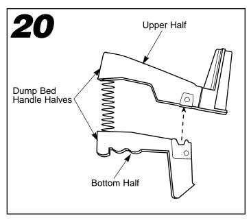
Re-assemble the two halves of the dump bed handle.
