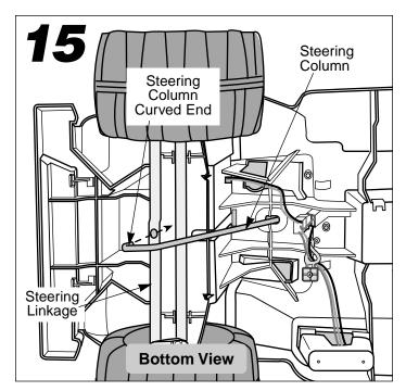
• Fit the curved end of the steering column into the hole in the steering linkage.
