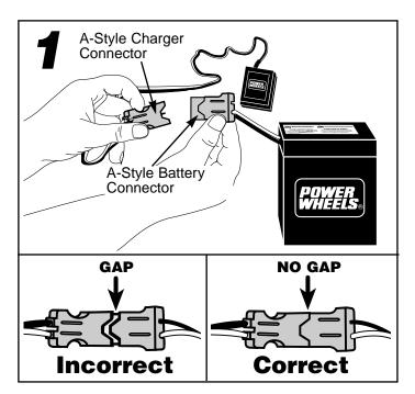
Plug the charger and battery connectors together.
