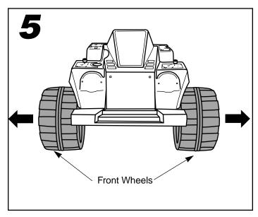
· Slide the front wheels off the front axles.
