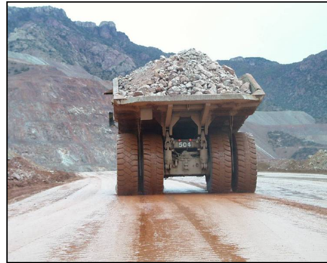
Excess cross fall
