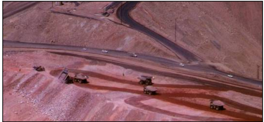
Good dump area – keeps tire cuts at minimum
