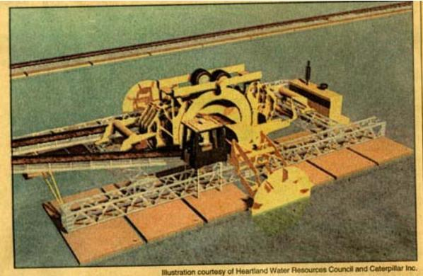
A computerized depiction of the river dredge designed by Caterpillar Inc. engineers shows the 20-foot wheel dredge and the conveyor belt to remove silt from rivers. If it works as planned, it would be more efficient and cheaper than current dredging technology. A new company is being formed to build and test this dredge. A DeKalb-area competitor is working on a similar design.
