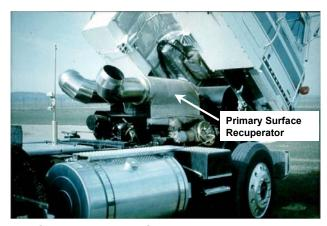
Caterpillar T-450 Gas Turbine Installed in International Transtar Highway Tractor
