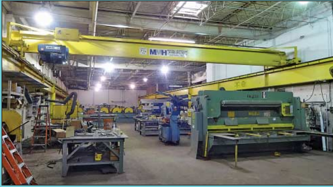
7.5 Ton X 50' Approx. Span X 200' Long Macko Material Handling Single Girder Free-Standing Overhead Bridge Crane
