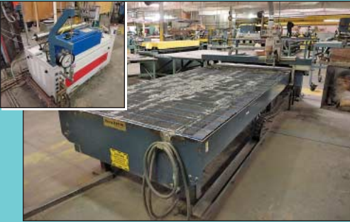
5' X 10' Lockformer Model 1600-WJ CNC Water Jet Insulation Cutter
