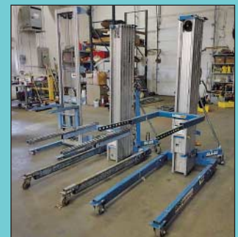
(2) Genie Model SL-25 Duct Lifts
