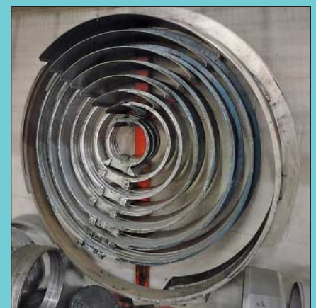
Large Quantity of Spiral-Helix Tube Forming Sets Including; 10", 12", 14" Wide Sets Up to 60" Diameter
