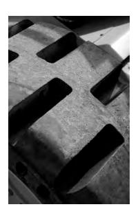
The OTR design has a block pattern that provides a degree of traction in applications where debris is not an issue.
