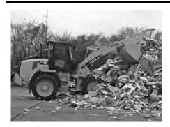
Cat Flexport tires for Compact Wheel Loaders are a 1-piece tire / rim design and are available in directional construction, smooth and OTR tread patterns.
