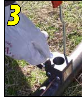
3 Place metal disc in bottom of mold.
