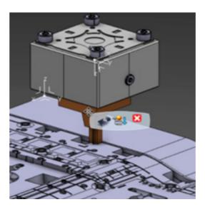
One of the most time-consuming tasks for the tool designer is defining the forming-related elements of the part: core/cavity blocks, lifter/slider heads, sub-inserts, and electrodes.
