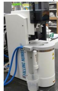
5. Place stirrers into 6. Place tubes in FN machine, tubes in white holder. stirs and heats for 60 sec
