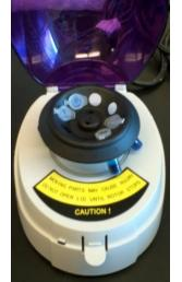
7. Place tubes in centrifuge so that it's balanced. Spin for ~30 seconds.
