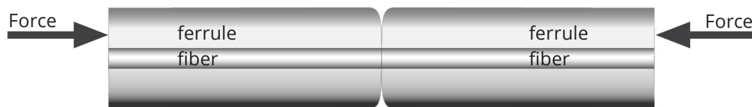
Figure 9: PC-PC mating with pressure applied deforming the ferrule and fibers make contact.
