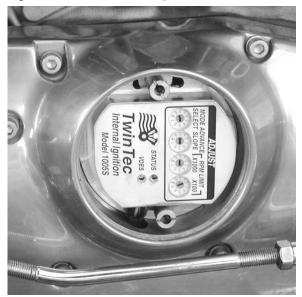
8. Refer to the appropriate wiring diagram. Use the dual fire hookup shown in Figure 4 if you have an OE coil or other coil with two primary terminals. Use the single fire hookup in Figure 5 if you are installing an aftermarket coil with three primary terminals. Use appropriate crimp terminals for coil and VOES hookup. With the exception of the tachometer and rear coil section (single fire only), standard H-D® wire color codes are used. Tape up any unused wires.
