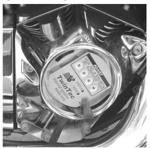
Figure 3A - Finished Big-Twin® Installation
