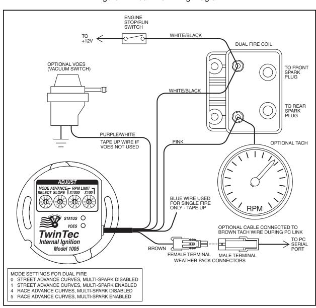
Figure 4 - Dual Fire Wiring Diagram
