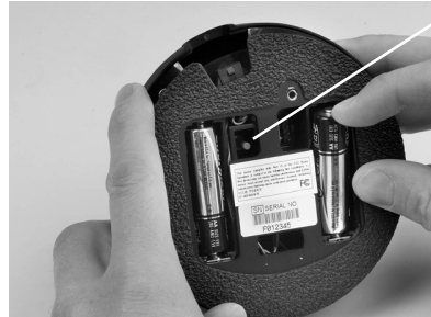
Look for blinking communications light.
