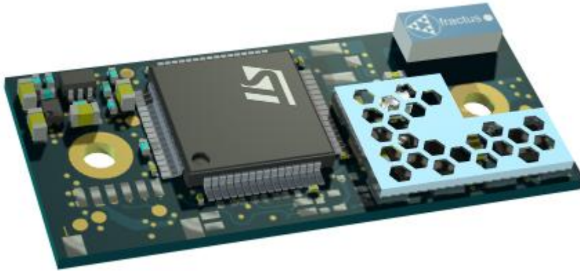
Figure 1: cB-OBS410i-04 OEM Serial Port Adapter with internal antenna
