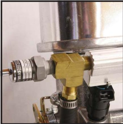
filter. A new tank bung is provided with a 1/2" hose barb as well. The filter goes inline between the tank and pump, and is marked with an arrow for direction of flow. Make sure it points the correct way. Two "P" clamps are used to attach the pump to any flat surface. Mount the pump below tank level and in the horizontal position. Make sure there are no kinks in the hose. Connect the discharge end to the fuel line in the chassis.
