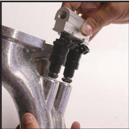
assembly, some fuel rail hold downs need to be used. Refer to pictures to correctly assemble the hold down assemblies.
