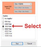
Tip: Leave the amplifier in-line, but switched off, and de-selected in the software, for discharge rates less than 100 watts (An amplifier is bypassed and disabled whenever it is powered off).
