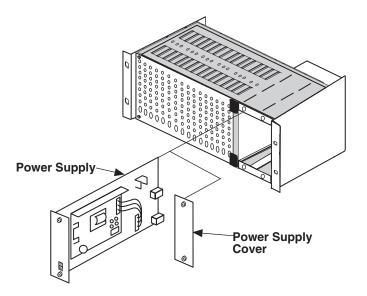
Figure 2-3. Power Supply Installation
