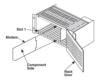
Figure 2-1. Modem Installation
