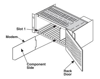
Figure 2-1. Modem Installation
