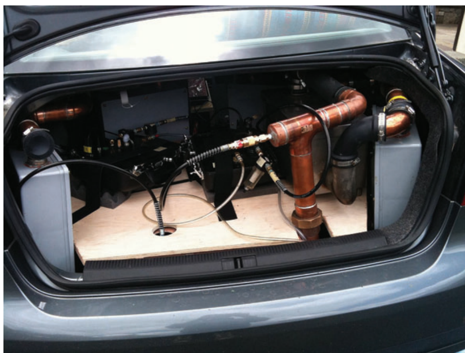
Figure 1 - a prototype of the Strataclear technology installation in the trunk of the test vehicle. Pipes and cables in the car trunk are only for testing purposes, performed using the computerized industry standard, five gas analyzers, complemented with On Board Diagnostics version II reading of the engine data. This is typically performed by the car servicing station, to diagnose problems and collect data. The analyzers and part of the exhaust gas conduits are visible in the trunk.
