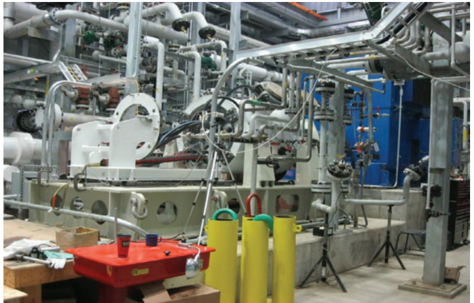
Figure 1 - Ramgen 8 MW, 10:1 pressure ratio CO 2 compressor being assembled for test on the Dresser-Rand dedicated closed-loop CO 2 test facility in Olean, NY, USA
