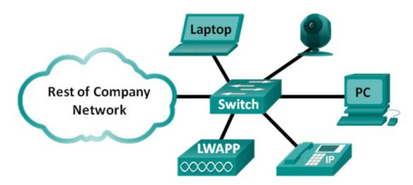
a. Company A requires a replacement access switch in the wiring closet. The company requires the switch to support VoIP and multicast, accommodate future growth of users and increased bandwidth usage. The switch must support a minimum of 35 current users and have a high-speed uplink. List a few of models that meet those requirements.
