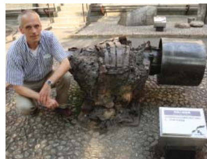
Roel at the memorial site of the 1923 Great Kanto earthquake. This devastating earthquake triggered fires that caused much loss of life, and which were sufficiently intense to melt the iron in the electro-motor shown in the photo.
