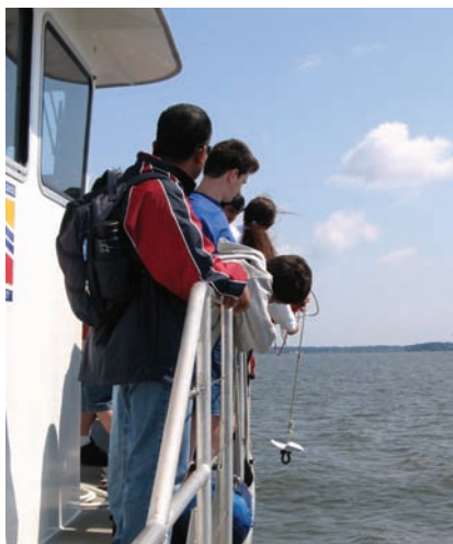
Boy Scouts deploy a Secchi disk from the R/V Fay Slover to measure visual water clarity.
