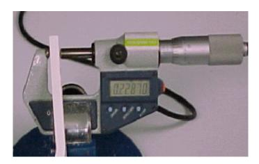
The student learns about the physical properties of the CIPP and what the inspector needs to do to verify that the installed product meets the specification requirements
