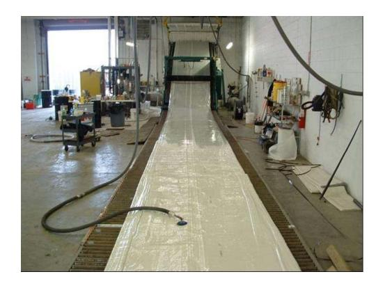
The student learns about the process of impregnating the resin material into the dry tube in a factory environment
