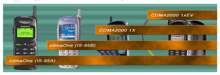
cdmaOne<sup>™</sup> identifies 2G and 2.5G cellular, PCS and wireless local loop (WLL) services based on the IS-95A and IS-95B CDMA air interface standards. IS-95A supports data delivery up to 14.4 kbps while IS-95B offers up to 115 kbps.
