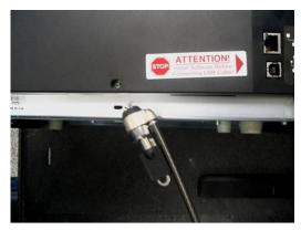
The HDPii Printer has a Security Lock Slot located in the back lip of the metal chassis to accommodate a standard laptop security lock.
