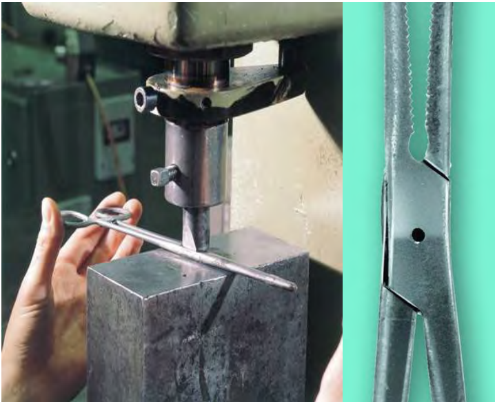
Figure 18 – Pressing the Individual Parts of a Two-Part Instrument Together
