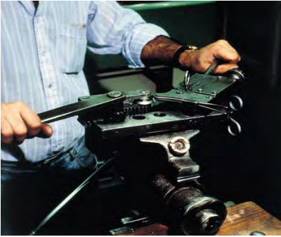
Figure 21 – Bending the Mouth of an Atraumatic Clamp
