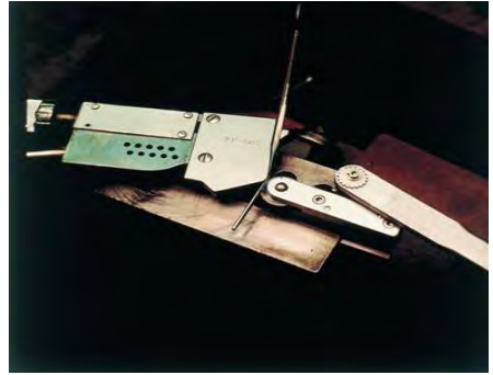
Figure 21 – Bending the Mouth of an Atraumatic Clamp
