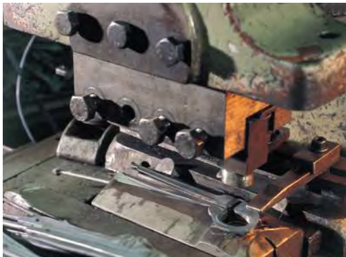
Figure 11 – Deburring/Dulling of Forged Raw Parts
