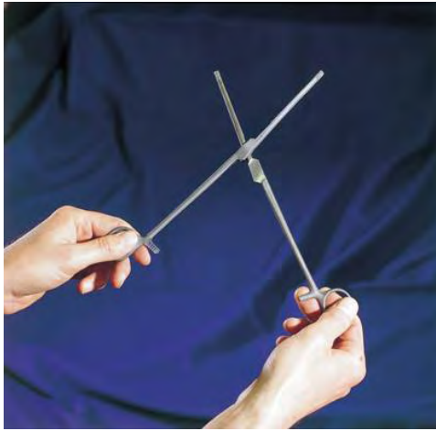
Figure 17 – Inserting the Male Component of a Clamp Joint into the Female Component
