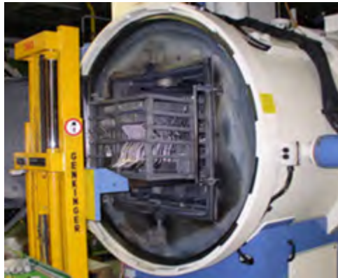
Figure 24 – Vacuum Hardening Furnace
