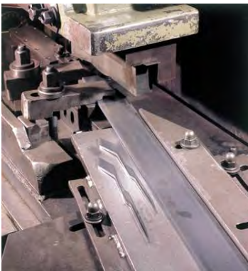
Figure 9 – Splitting Machine and Unattached Part Cut from the Steel Strip
