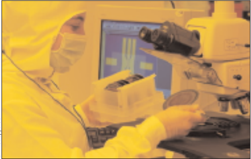
Observation of a silicon wafer using an optical microscope.
