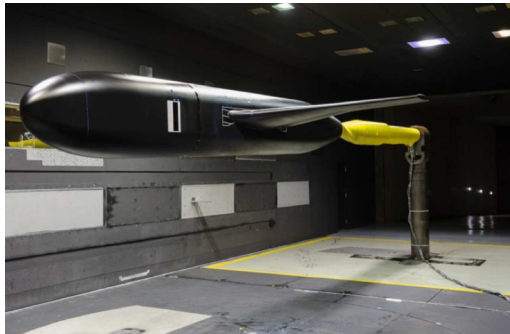
FIGURE 1. Experimental setup of the NASA Juncture Flow at NASA Langley 14- by 22-foot Subsonic Wind Tunnel.
