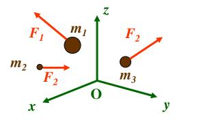
$M\vec{a}_{com} = m_1\vec{a}_1 + m_2\vec{a}_2 + m_3\vec{a}_3 + \dots + m_n\vec{a}_n$ We apply Newton's second law for the *i*-th particle:  $m_i\vec{a}_i = \vec{F}_i$  Here  $\vec{F}_i$  is the net force on the *i*-th particle  $M\vec{a}_{com} = \vec{F}_1 + \vec{F}_2 + \vec{F}_3 + \dots + \vec{F}_n$
