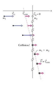
One Dimensional Inelastic Collisions In these collisions the linear momentium of the colliding objects is conserved  $\rightarrow \vec{p}_{1i} + \vec{p}_{2i} = \vec{p}_{1f} + \vec{p}_{2f}$  $m_1 \vec{v}_{1i} + m_1 \vec{v}_{2i} = m_1 \vec{v}_{1f} + m_1 \vec{v}_{2f}$
