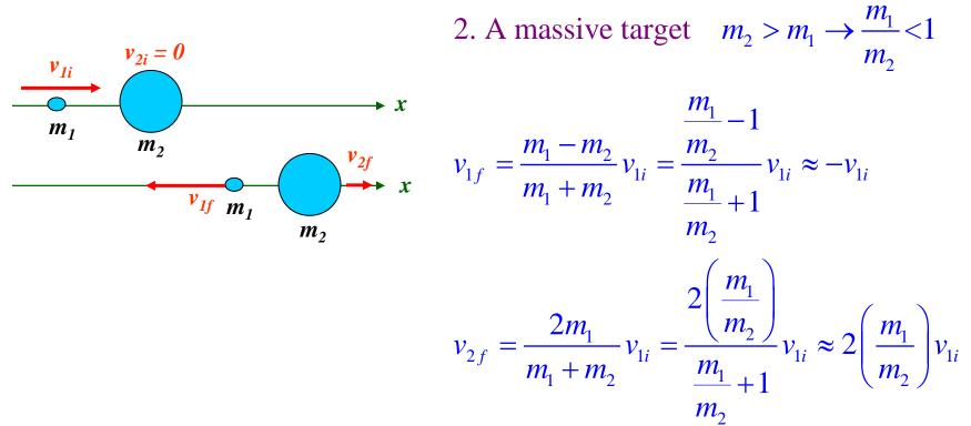
Body 1 (small mass) bounces back along the incoming path with its speed practically unchanged.
