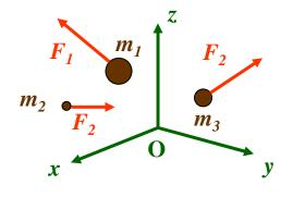
Newton's Second Law for a System of Particles Consider a system of *n* particles of masses  $m_1, m_2, m_3, ..., m_n$ and position vectors  $\vec{r_1}, \vec{r_2}, \vec{r_3}, ..., \vec{r_n}$ , respectively. The position vector of the center of mass is given by:
