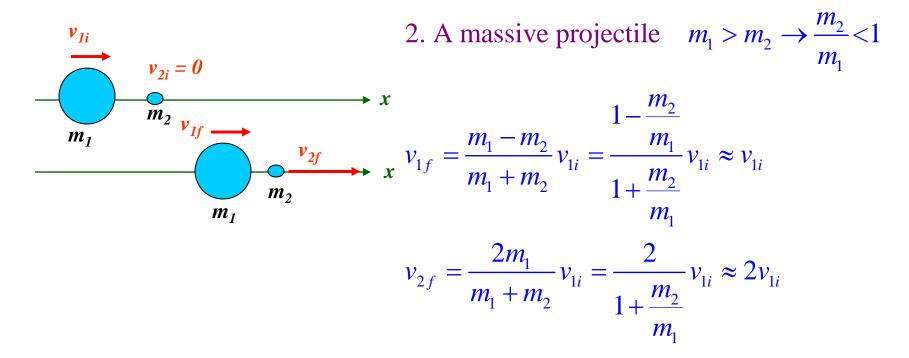
Body 1 (large mass) keeps on going scarcely slowed by the collision . Body 2 (small mass) charges ahead at twice the speed of body 1
