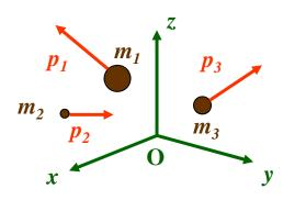
The Linear Momentum of a System of Particles In this section we will extedend the definition of linear momentum to a system of particles. The *i*-th particle has mass  $m_i$ , velocity  $\vec{v}_i$ , and linear momentum  $\vec{p}_i$
