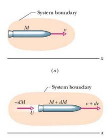
Using the conservation of linear momentum we derived the equation of motion for the rocket
