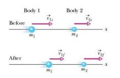
Momentum and Kinetic Energy in Collisions Consider two colliding objects with masses  $m_1$  and  $m_2$ , initial velocities  $\vec{v}_{1i}$  and  $\vec{v}_{2i}$  and final velocities  $\vec{v}_{1f}$  and  $\vec{v}_{2f}$ , respectively
