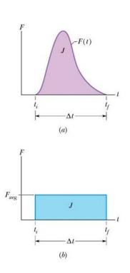
Consider the collision of a baseball with a baseball bat The collision starts at time  $t_i$  when the ball touches the bat and ends at  $t_f$  when the two objects separate The ball is acted upon by a force  $\vec{F}(t)$  during the collision The magnitude F(t) of the force is plotted versus t in fig.a The force is non-zero only for the time interval  $t_i < t < t_f$  $\vec{F}(t) = \frac{d\vec{p}}{dt}$  Here  $\vec{p}$  is the linear momentum of the ball
