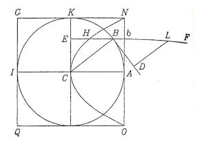
F(B), F(b) := force acting in B or b, resp., |BC| = 1, |LB| = 1. F(B) : F(b) = LD : LB = BE : BC.  $F_e :=$  component of F acting in direction e; therefore  $F_e(B) : F_e(b) = BE^2 : BC^2$ . Summation of forces: Define H on the line EF by
