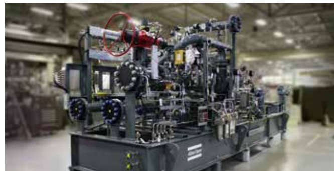
An Atlas Copco fuel gas booster
