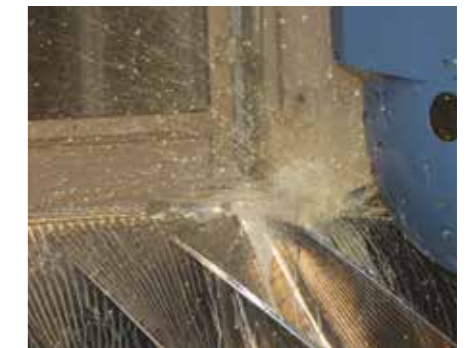
Inside the multi-skill machine: the milling process
