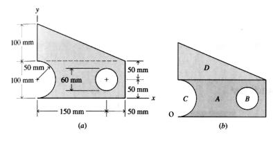
$I_x = (200 \text{ mm})(100 \text{ mm})^3/12 = 16.667 \text{ x } 10^6 \text{ mm}^4$  $I_y = (200 \text{ mm})^3 (100 \text{ mm})/12 = 66.667 \text{ x } 10^6 \text{ mm}^4$
