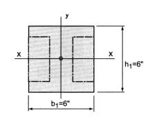
Determine the moments of inertia about the centroid of the shape.
