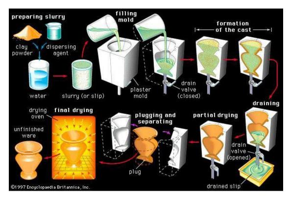
Figure 1: Schematic showing the steps used in slip casting. First the slip is prepared by mixing the ceramic powder with a liquid. Next the slip is poured into the mold which absorbs the liquid out of the slip leaving a thin wall of powder along the mold wall. The access slip is removed and the green body can then be removed from the mold. Finally, your part is placed in a furnace to be sintered into the final dense object. (https://www.britannica.com/technology/traditional-ceramics)
