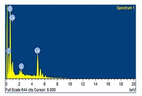
Fig. 3. EDX of cerium oxide nanoparticles
