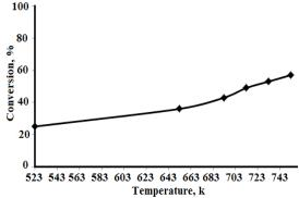
Fig. 4. Conversion of methanol over 0.5 g of cerium oxide, 5 h' TOS, 20 mL/min of O, and N, mixture
