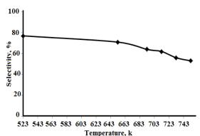
Fig. 5. Selectivity of formaldehyde over 0.5 g of cerium oxide, 5 h 'TOS, 20 mL/min of O<sub>2</sub> and N<sub>2</sub> mixture
