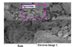
Fig. 2. SEM of cerium oxide nanoparticles
