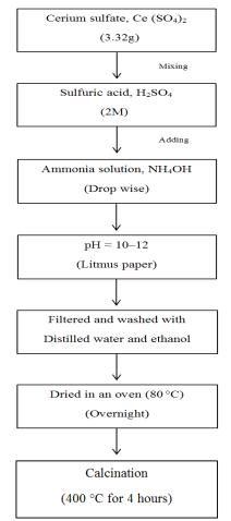
Schematic diagram for the synthesis of CeO<sub>2</sub> nanoparticles
