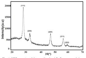
Fig. 1. XRD spectra of the synthesized  $\text{CeO}_2$  nanoparticles
