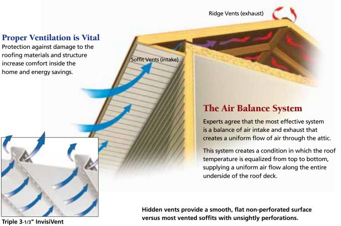
Triple 3-1/3" InvisiVent offers at least 50% more ventilation than most standard vinyl soffit, providing more than 10" of net-free intake area.
