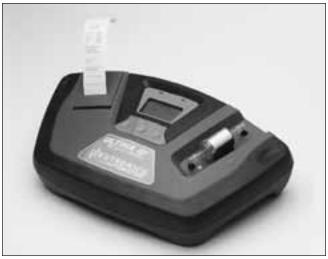
While not required by federal law, the use of a refrigerant identifier is strongly recommended. It can help you determine if a vehicle contains contaminated refrigerant that you would not want inside your recovery machine. Identifiers can also provide an accurate indication concerning the amount of air that may be in an A/C system or storage tank. Some state or local laws may require their use.
