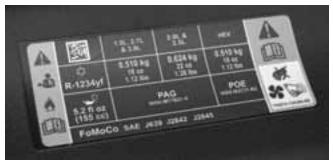
A vehicle's A/C system information label lists the type of lubricating oil that the system requires.
