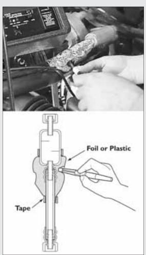
To help confirm a suspected leak, place aluminum foil or plastic wrap and tape it around the connection or component. If there truly is a leak, after a few minutes, refrigerant should accumulate inside the plastic wrap or foil. Make a small hole in the foil or wrap at the lowest point possible and place your leak detector probe at the hole. The detector will indicate "refrigerant found" if a leak is actually present.
