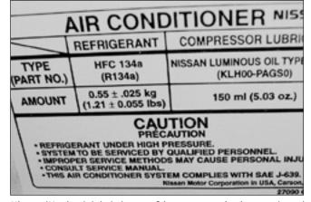
Nissan (Maxima) label shows refrigerant capacity in pounds and kilograms, to two decimal places, and a tolerance to three decimal places.
