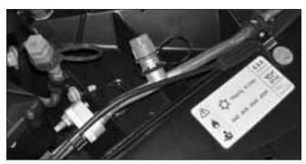
The caps are the service ports' primary seal against refrigerant leakage. Always make sure that every service port has one in place.
