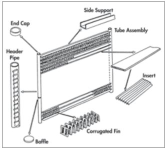
The condensers used in HFC-134a systems are more efficient than the ones that were used in CFC-12 systems. The 3/8-inch tube-and-fin condenser shown on the left diagram is an example of the type that was used for many years in CFC-12 systems. The parallel flow/multi-flow condenser on the right diagram is representative of the type of condensers used in most HFC-134a systems.
