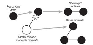
A free oxygen atom breaks up the chlorine monoxide molecule. The chlorine atom is then free to repeat the process.
