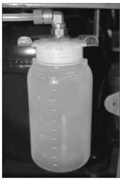
Here is a typical recovery machine's oil recovery reservoir. It should be emptied before each recovery operation, then checked when recovery is completed to see how much (if any) oil was removed from the system during recovery. If oil was removed, that same quantity of fresh new oil of the type the system requires must be reinstalled in the system before it is put back into operation.
