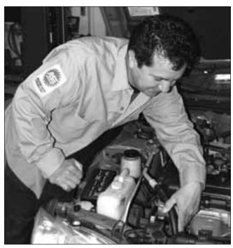
Before connecting service equipment, always perform a visual inspection of the A/C system to spot any obvious problems.
