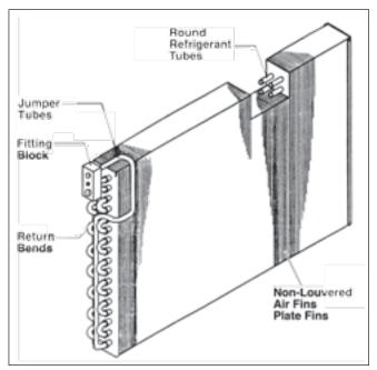
The most noticeable changes however, were redesigned condensers, which incorporated increased airflow to reduce system pressures at low speed operation and city traffic conditions. In general, condenser performance for HFC-134a systems increased by approximately 30% over that of CFC-12 systems, which resulted in comparable performance between the two refrigerants.
