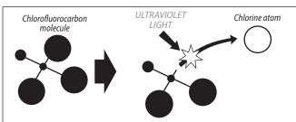
1) In the upper atmosphere, ultraviolet light breaks off a chlorine atom from a chlorofluorocarbon molecule.
