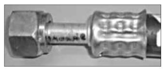
Assembly crimped, rotated and recrimped.
