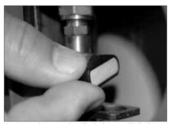
You can use the recovery/recycling/recharge machine's air purge valve to purge excess air from recycled refrigerant. Let the air out, and watch the pressure gauge on the machine's panel. When the gauge reading reaches the appropriate number in the table (based on the ambient temperature), close the purge valve. The recycled refrigerant now does not contain an excessive amount of air, and can be reused to recharge an A/C system.
