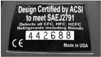
Typical leak detector certification label. It shows that this leak detector meets the minimum performance requirements outlined in SAE standard J2791.
