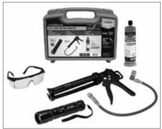
A typical UV dye leak detection kit contains dye, a dye injector (or some other type of tool to introduce dye to a system), a UV flashlight, and the correct goggles for the dye being used. Always wear the goggles to protect your eyes from the UV light. This kit also contains a special cleaner to remove traces of the dye after the leak is repaired.
