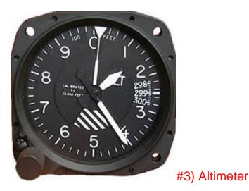
The Altimeter measures the Altitude or height of the aircraft above Sea Level. Remember, ground elevation varies widely, so the Altimeter reading does not measure height about the Ground, but instead above Sea Level. The Pilot must be aware of the Ground elevation, to then calculate the height of the airplane above the Ground.
