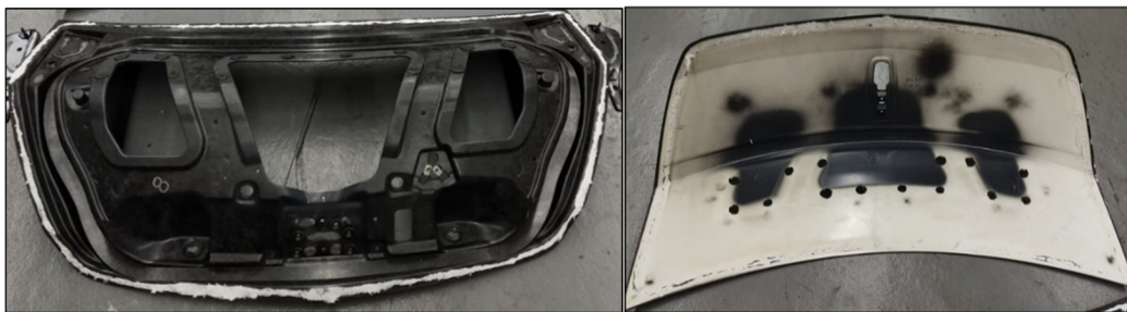
Figure 11. Decklid assembly teardown for validation of adhesive placement and bond strength
