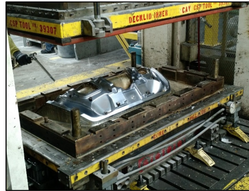
Figures 8 and 9. Decklid inner charge pattern and Lincoln MKS decklid inner molding tool.
