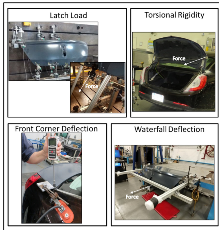
Figure 12. Physical testing of prototype decklid assemblies.
