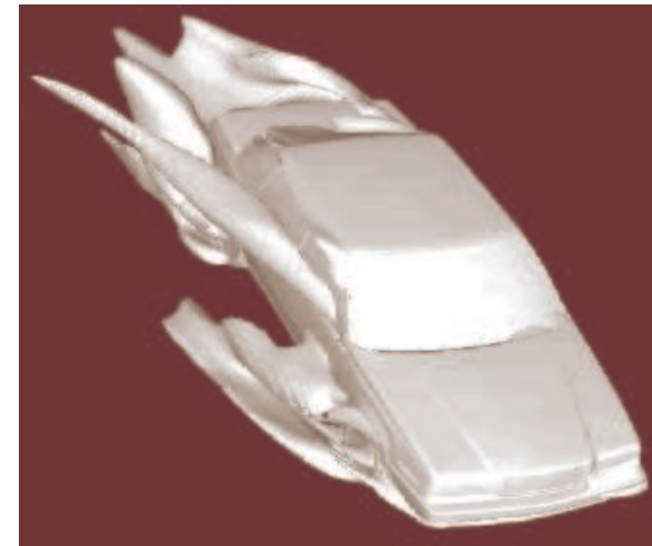
Representation of the wake with yaw = 30 degrees
