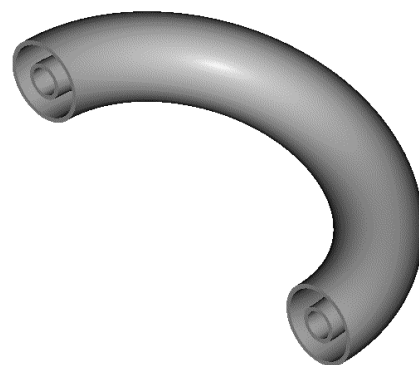
Fig.1(b) Close-up of double pipe coil
