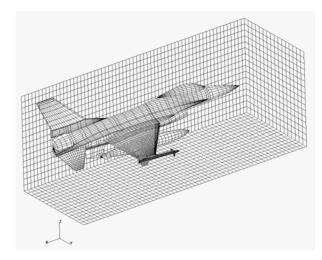
Figure 13. TRANAIR Global Grid, Contract Test Case
