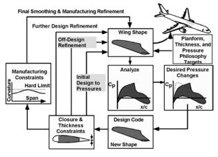
Figure 23. Iterative/Inverse Design Process
