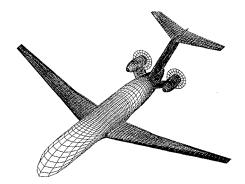
Figure 17. Surface Grid on an Advanced Propfan Transport
