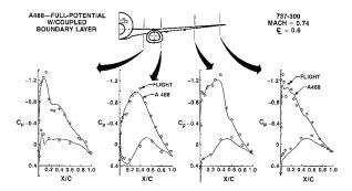
Figure 12. Comparison with Flight Pressure Distributions—737-300
