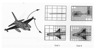
Figure 14. TRANAIR Grid Refinement, Contract Test Case
