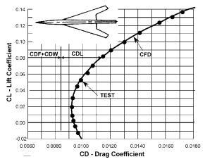
Figure 6. Early Boeing SST Test Versus CFD Comparison—733-290 - Mach=2.7
