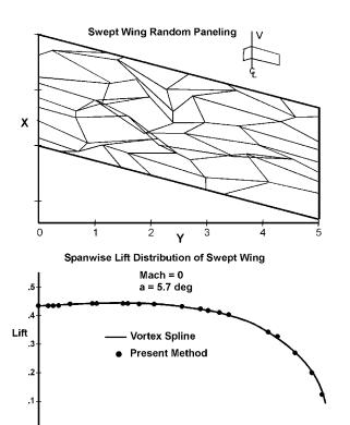
Figure 9. Swept Wing Random Paneling Test
