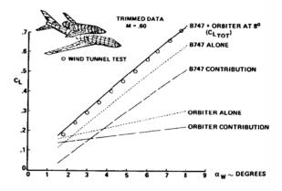
Figure 8. B747-Orbiter Lift Coefficient
