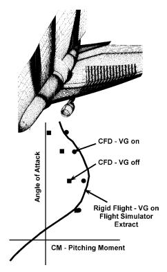
Figure 20. Effect of Vortex Generators on Pitching Moment
