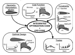
Figure 24. TRANAIR Optimization-Based Aerodynamic Design
