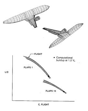
Figure 10. 737-300 High-Lift Lift/Drag Comparison
