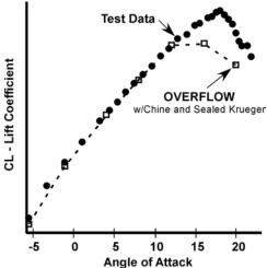
Figure 21. OVERFLOW Solution on a High-Lift Configuration
