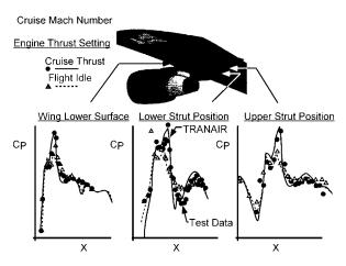
Figure 16. CFD Simulation of Installed Engine Exhaust Effects
