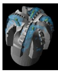
Flow of lubricating mud over drill bit
