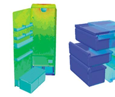
Surface-heat-flux plots of the No-Frost refrigerator and freezer compartments helped BOSCH-SIEMENS engineers to optimize the location of air inlets.
