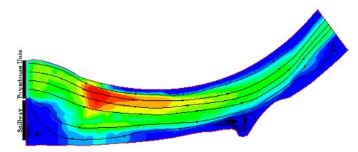
Total Discharge = 125,000 cfs (no flow through spillway)
