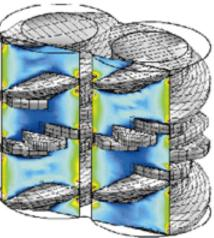
Shear rate distribution in twinscrew extruder simulation
