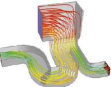
Flow pathlines colored by pressure quantify head loss in ductwork Source: internet
