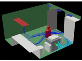
Particle traces of copier VOC emissions colored by concentration level fall behind the copier and then circulate through the room before exiting the exhaust.
