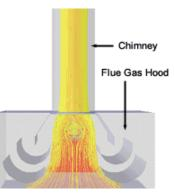
Pathlines from the inlet colored by temperature during standard operating conditions
