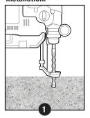
Using the proper drill bit size, drill a hole into the base material to the required depth. The tolerances of the drill bit used should meet the requirements of ANSI standard B212.15
