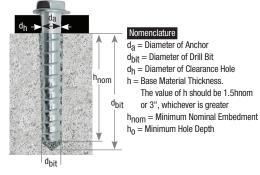
Screw-Bolt ™ + anchor detail
