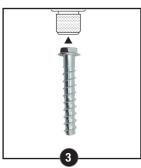
Select a torque wrench or powered impact wrench and do not exceed the maximum torque, Tinst, max or Timpact, max respectively for the selected anchor diameter and embedment. Attach an appropriate sized hex socket/driver to the impact wrench. Mount the screw anchor head into the socket.
