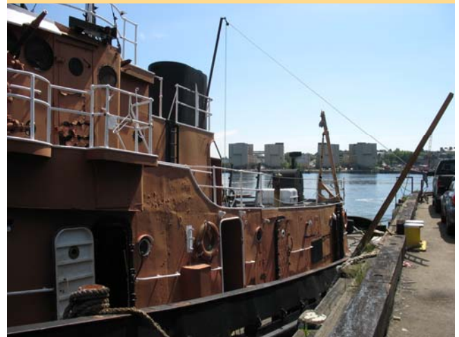
Exterior Rust build-up
