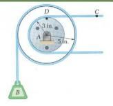
Cable *C* has a constant acceleration of 9  $in/s^2$  and an initial velocity of 12 in/s, both directed to the right.
