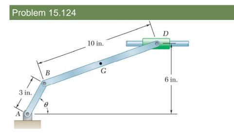
Arm *AB* has a constant angular velocity of 16 rad/s counterclockwise. At the instant when  $\theta=90^{\circ}$ , determine the acceleration (a) of collar *D*, (b) of the midpoint *G* of bar *BD*.
