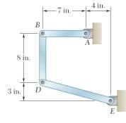
Knowing that at the instant shown bar *AB* has a constant angular velocity of 4 rad/s clockwise, determine the angular acceleration of bars *BD* and *DE*.
