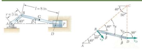
What happens to the location of the instantaneous center of velocity if the crankshaft angular velocity increases from 2000 rpm in the previous problem to 3000 rpm?
