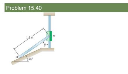
Collar *B* moves upward with a constant velocity of 1.5 m/s. At the instant when  $\theta$ =50°, determine (a) the angular velocity of rod *AB*, (b) the velocity of end *A* of the rod.
