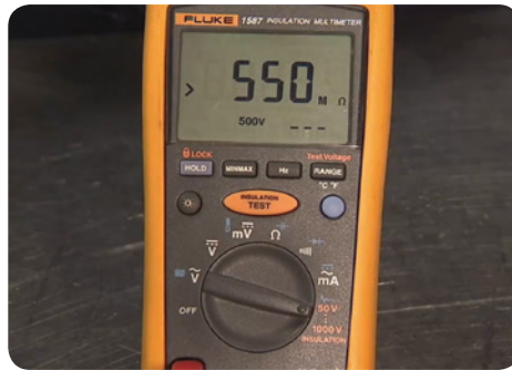
Set the meter to the 500V range.
