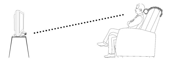
Place the transmitter on a stable flat surface so the front of the transmitter can be pointed at the ChairSpeaker®, line of sight is required. Point the transmitter towards the ChairSpeaker®. Do not cover the lights on the front of the transmitter.
