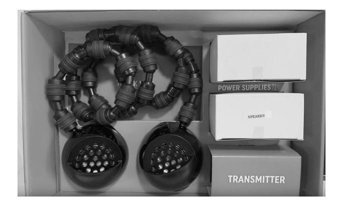
2 boxes with power adapters. One is for the speakers the other is for the transmitter.
