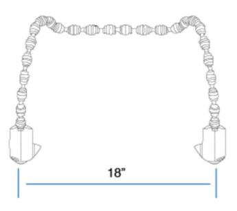
Make sure the side with the power inlet is in your right hand. Standing up facing your chair lay the ChairSpeaker® over the back of your chair and press the links hard against the chair to conform to the shape of your chair. Make sure some links go over the back. The rubber will hold onto your chair.
